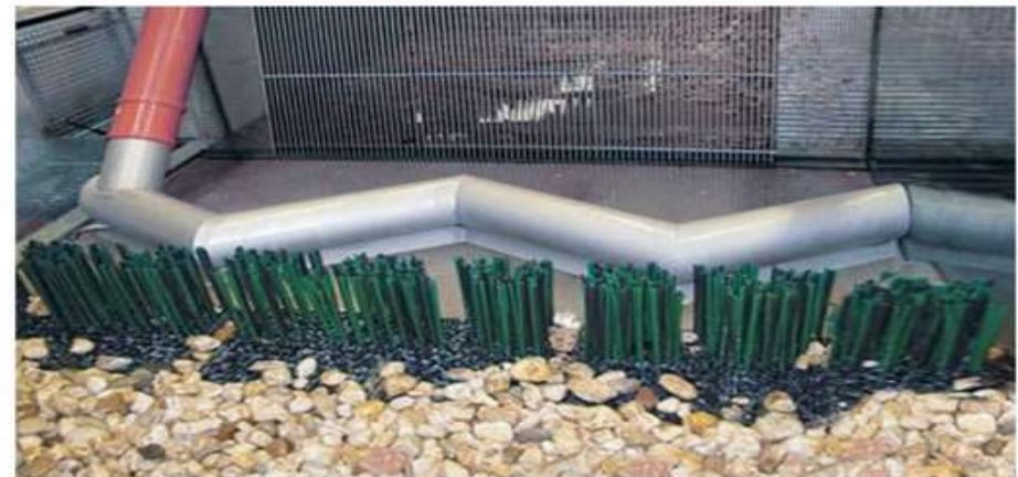
Fig. 5.16 Zigzag pipe in combination with bristle bundles installed in a model flume transversely to the screen ( www.klaw-gmbh.de ; accessed October 01, 2015)
